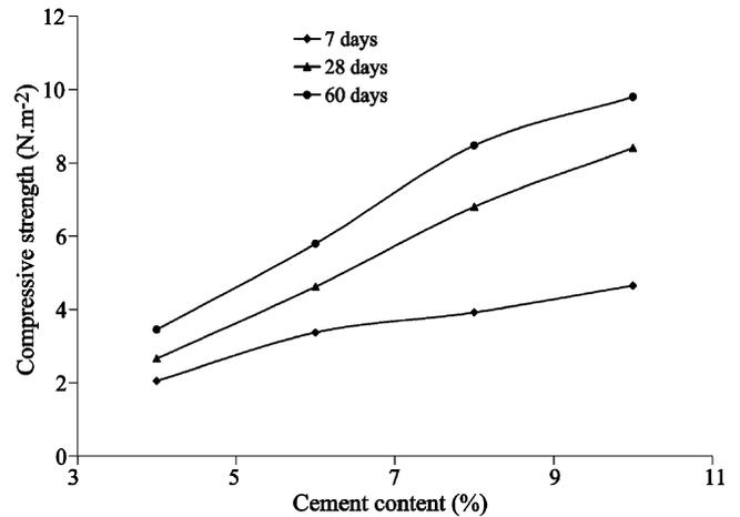
Fig. 7. Compressive strength as function of cement content.
