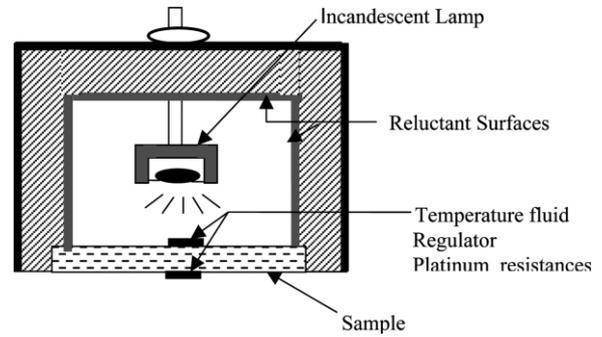
Fig. 3. Thermal diffusivity measurement apparatus.
