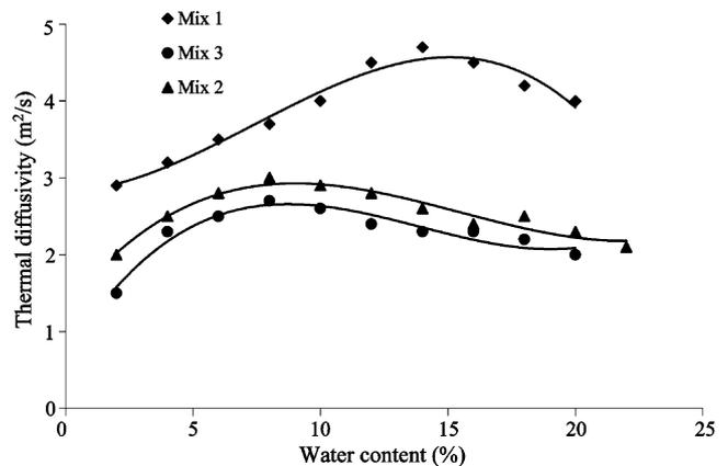
Fig. 5. Thermal diffusivity as function of water content.
