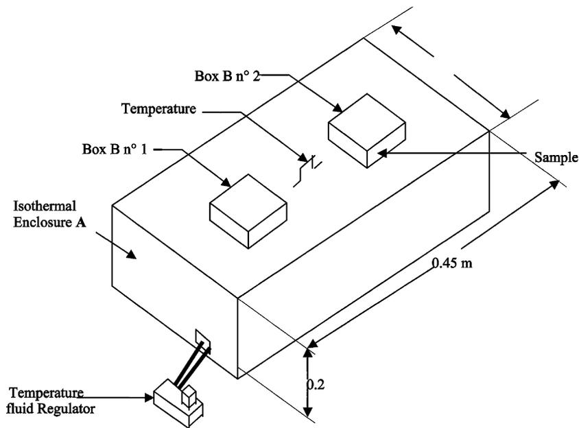
Fig. 2. Experimental setup of the box method.
