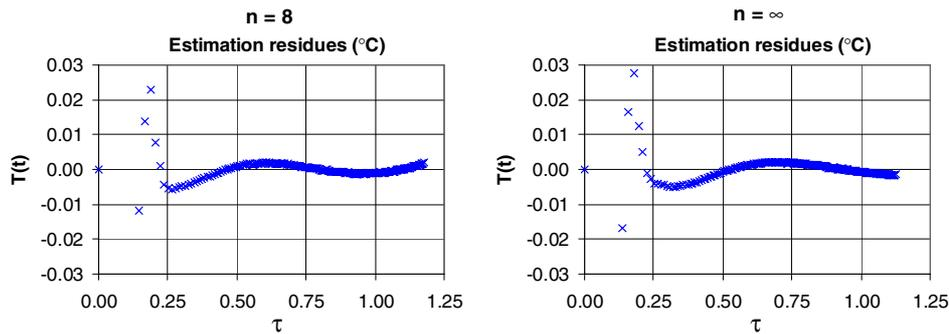
Figure 5. Estimation residues obtained with resistive ring numbers  $n = 8$  and  $n = \infty$ .
