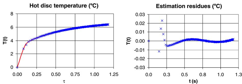
**Figure 4.** Hot disc temperature and estimation residues for a test on titanium TA6V.
