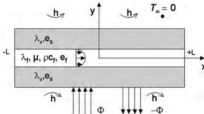
Figure 1. Geometry and structure of the flow.
