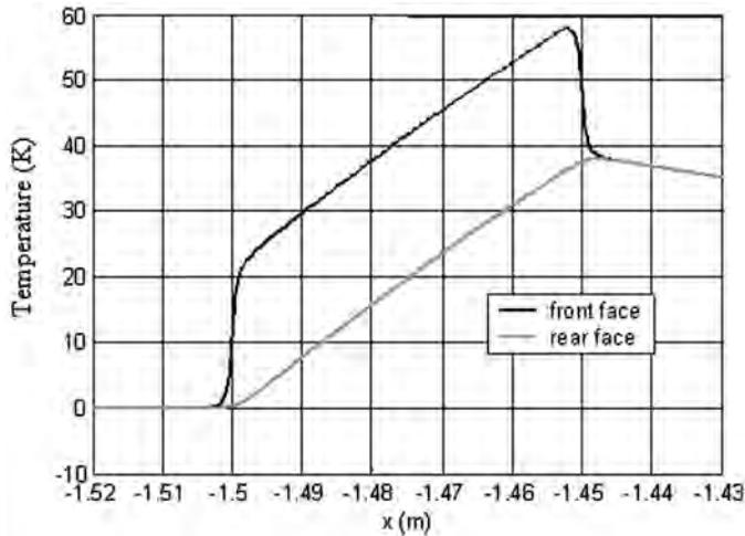
**Figure 4.** Local distribution of the front and rear temperatures over the heating region.
