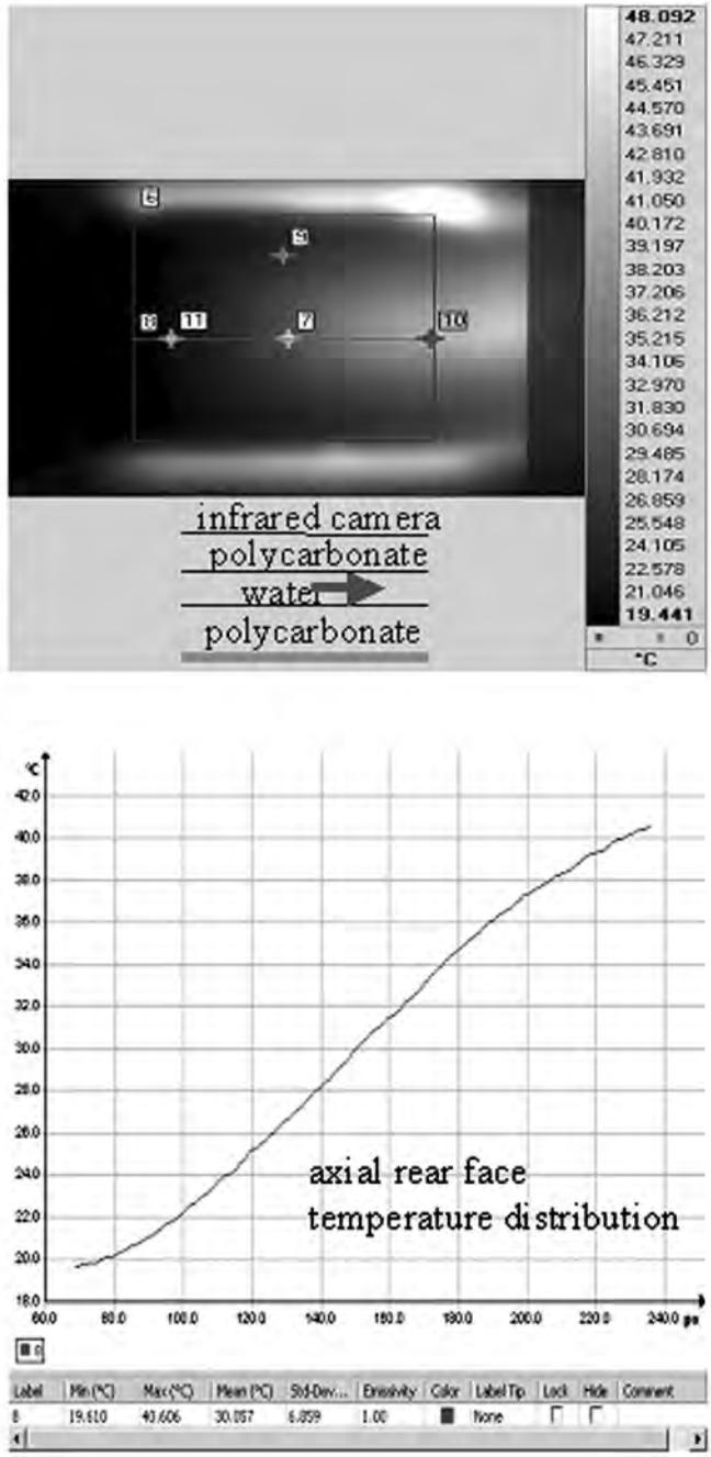
Figure 11. Infrared image and axial rear face temperature distribution.
