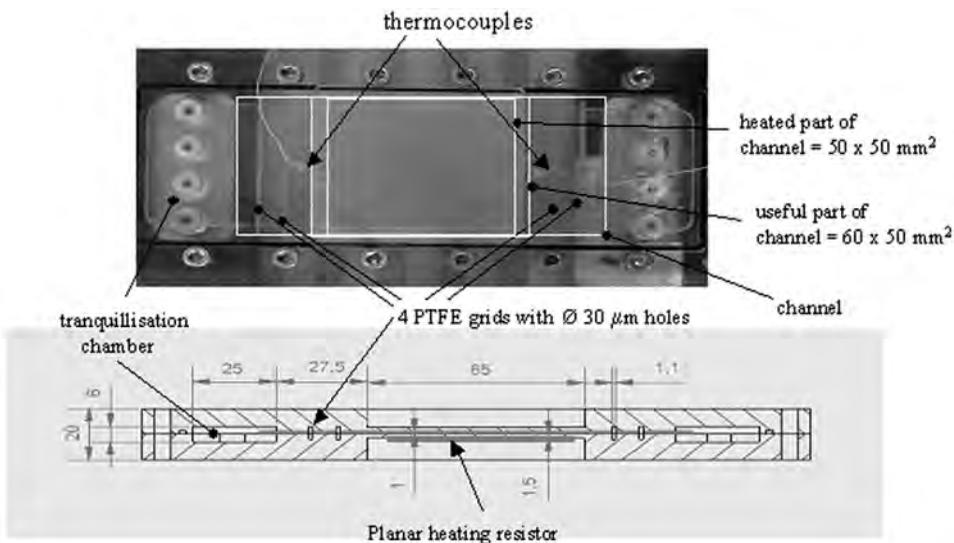
Figure 10. Realization of the mini-channel bench.
