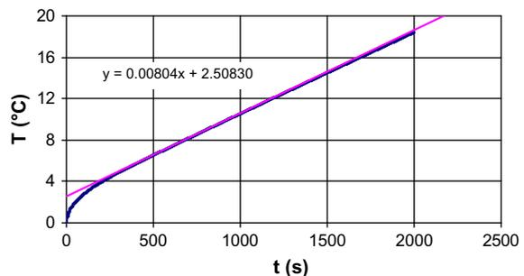
Fig. 6. Simulated curve  $T(t)$  calculated for  $e = 3$  cm,  $\lambda = 2$  W K<sup>-1</sup> m<sup>-1</sup>,  $\rho c = 2 \times 10^6$  J m<sup>-3</sup> K<sup>-1</sup>;  $e_i = 5$  cm,  $\lambda_i = 0.033$  W K<sup>-1</sup> m<sup>-1</sup> and  $\rho c_i = 40,000$  J m<sup>-3</sup> K<sup>-1</sup>.
