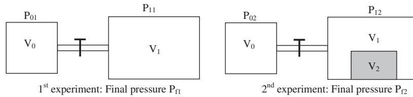
Fig. 3. Schema of the pycnometer calibration process.
