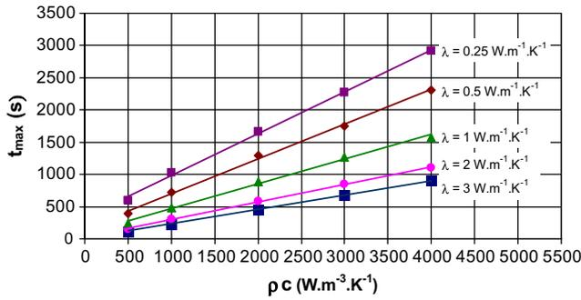
Fig. 7. Values of  $t_{\max}$  such as the deviation between the 1D and the 3D models is lower than 1% if  $t < t_{\max}$  (for  $h = 10 \text{ W m}^{-2} \text{ K}^{-1}$ ).
