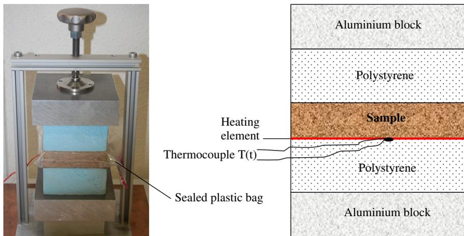
Fig. 5. View and schema of the experimental asymmetrical hot plate device.
