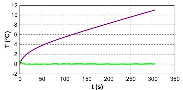
Fig. 9. Experimental and modeled hot plate temperature curves (+residues  $\times 10$ ) obtained with a PVC sample.
