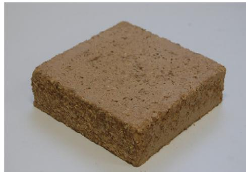
Fig. 1. View of millet waste used as insulating material and of a sample.
