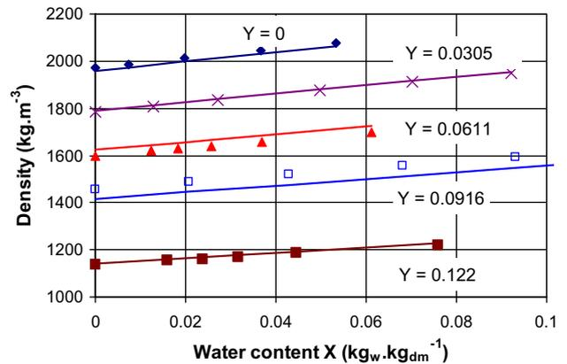
Fig. 8. Density  $\rho(X, Y)$  of laterite bricks with millet additive: theoretical values (lines) calculated with relation (21) and experimental values (points).
