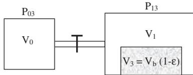
Fig. 4. Schema of porosity measurement method with the pycnometer.
