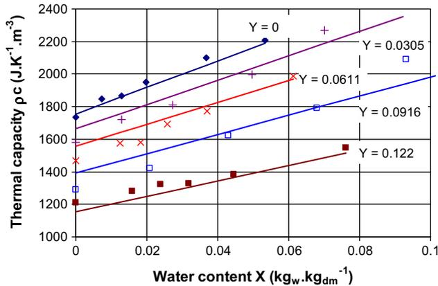
**Fig. 10.** Thermal capacity  $\rho c(X,Y)$  of laterite bricks with millet additive: theoretical values (lines) calculated with relation (22) and experimental values (points).
