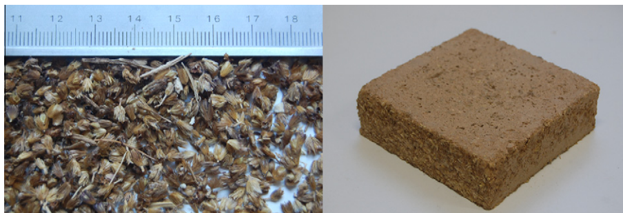
Fig. 1. Pictures of millet waste used as insulating material and of a sample.
