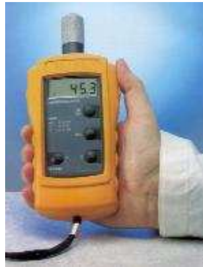
An example of a hygrometer based on a capacitance sensor
